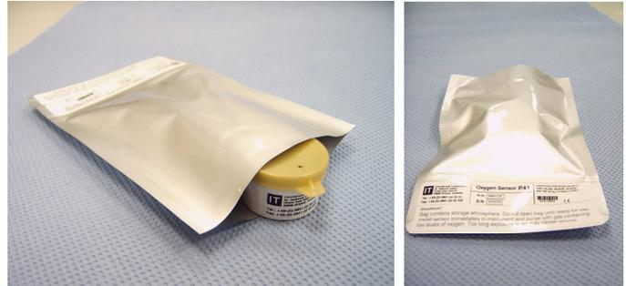
A spare cell should be carefully stored in an area that is not subject to large variations in ambient air temperature (between 5 to 25°C), and in such a way as to obviate any possibility of incurring damage. Never disturb the integrity of the cell package until the cell is to be actually used. If the cell package is punctured and air permitted to enter, the cell will immediately start to react to the presence of oxygen.
