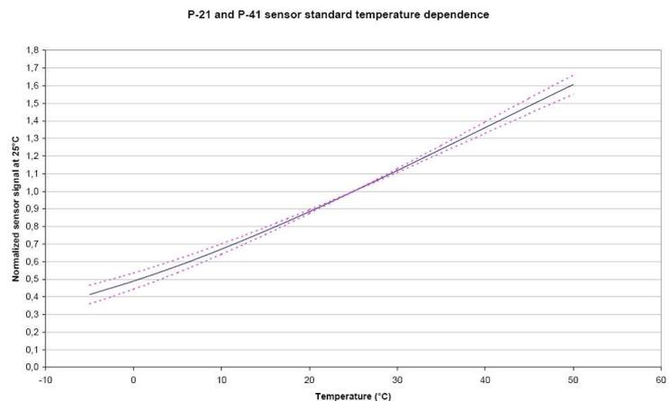
**Figure 3:** Standard temperature characteristic of trace oxygen cells
