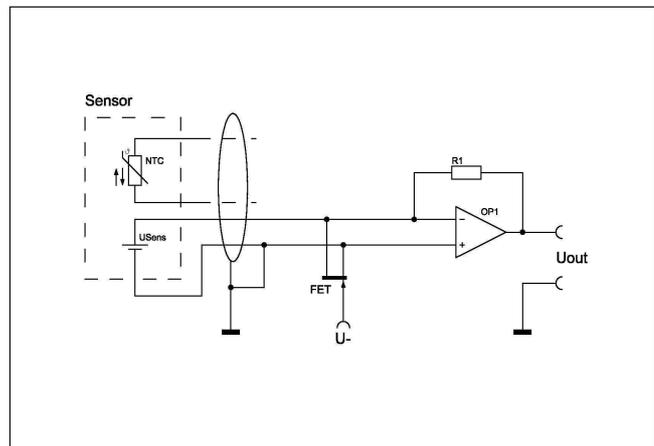
**Figure 5:** A typical electronic configuration of a first stage amplifier OP1.
