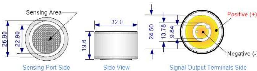
**Figure 2:** Three side view of P-type sensor. Do not block the venting holes to be seen on the Signal Output Terminals Side. Through this holes between the concentric metal foils the expansion membrane "breathes" when sudden pressure transients on the sensing area occur.
